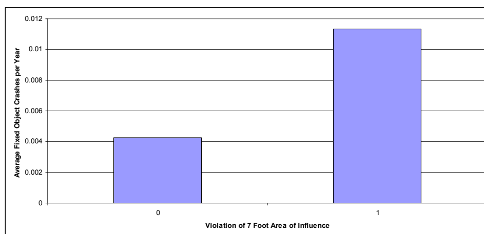
Figure 5-37. Violation of 7 ft area of influence in 15 m analysis
